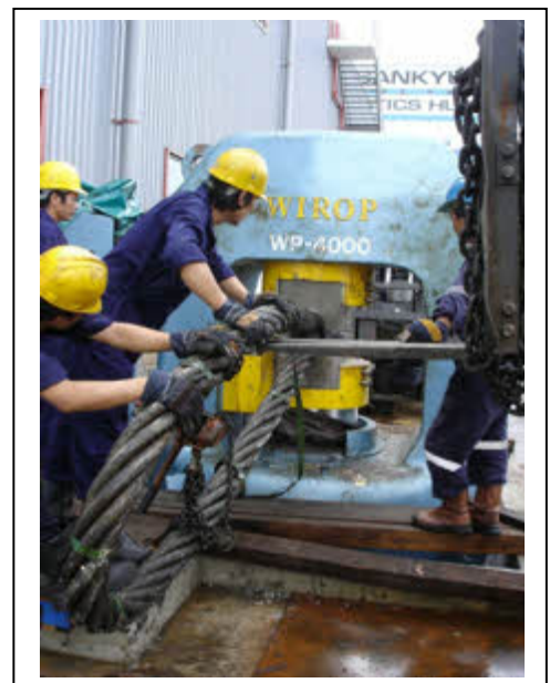
Above - Swaging a 6" (152mm) diameter KM SW AG E sling
